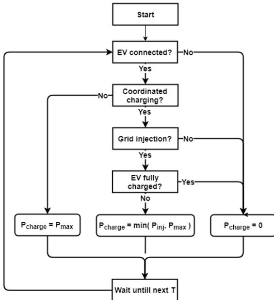
Fig. 7 Flowchart for coordinated charging – *Self-sufficiency*
