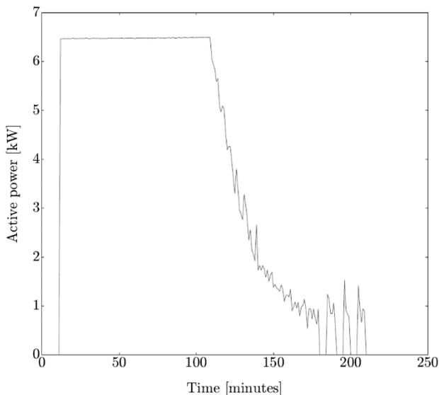
Fig. 6 Measured charging profile of the Nissan e-NV200
