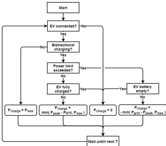
Fig. 9 Flowchart for bidirectional charging – PLR
