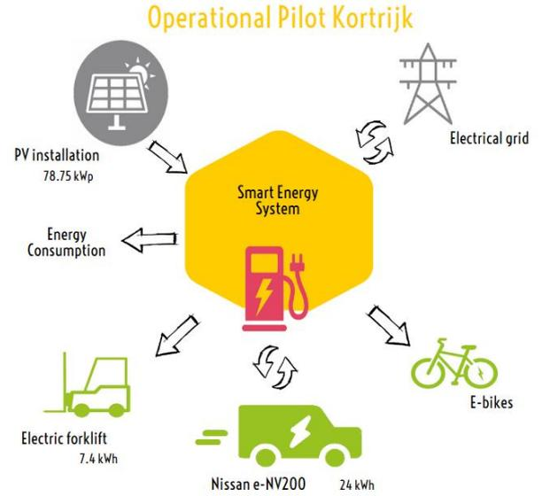
Fig. 4 Schematic of energy flows in Kortrijk pilot
