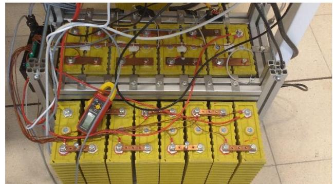
Fig. 10 Construction of 11 kWh stationary battery storage
